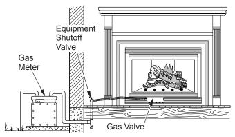
Figure 35 - Checking Gas Joints for Natural Gas Fireplace
